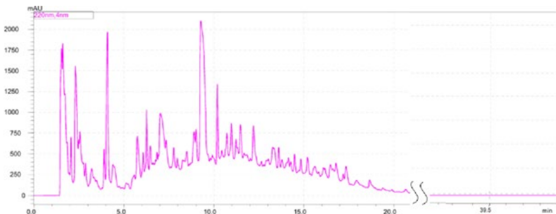
Figure 3: Isolation of peptides from the L. acidophilus IHMIA 9602 cell-free culture supernatant by reversed-phase chromatography. Column: Perkin-Elmer Quasar SPP C18, 2.7 \mu m, 4.6 x 100 mm. Eluent: 0–60 % ACN in 0.1% TFA over 22 minutes at 1.5 ml/min. 12 fractions.
