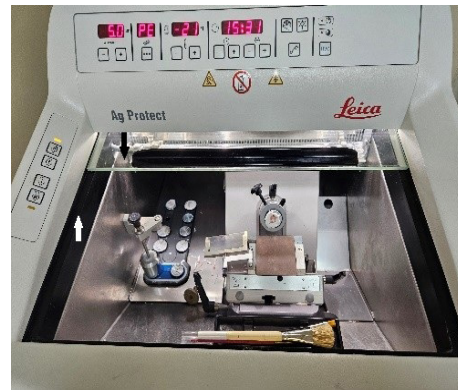
Figure 3: Cryostat with electronic monitor. Modern cryostat featuring digital temperature control and display.
