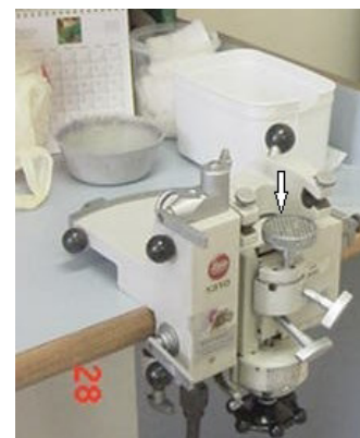
Figure 1: Portable freezing microtome. The white arrow indicates the freezing platform where the tissue is mounted.
