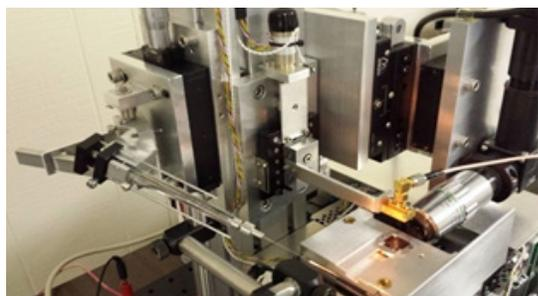
**Figure 1:** Vibratess spectrometer-Vibr2 with micro-syringe attached for accurate positioning of sample material. Micro-syringe is on the front left (not in dispensing position). Microfluidic chip with sample material is on the movable table (at right bottom of the picture) with the microdetector in a metal case (yellow) above it and the microscope objective behind it.
