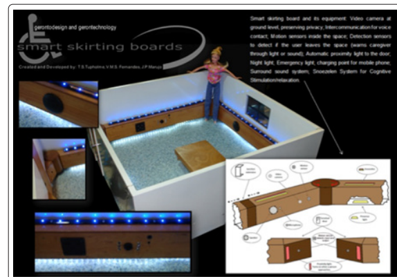
Figure 1: (A) SSB® and its equipment: Video camera at ground level, preserving privacy; Intercommunication for voice contact; Motion sensors inside the space; Detection sensors to detect if the user leaves the space (warns caregiver through light or sound); Automatic proximity light to the door; Night light; Emergency light; Charging point for mobile phone; Surround sound system; Snoezelen System -for cognitive stimulation/relaxation. (B) Room with a SSB® installed.
